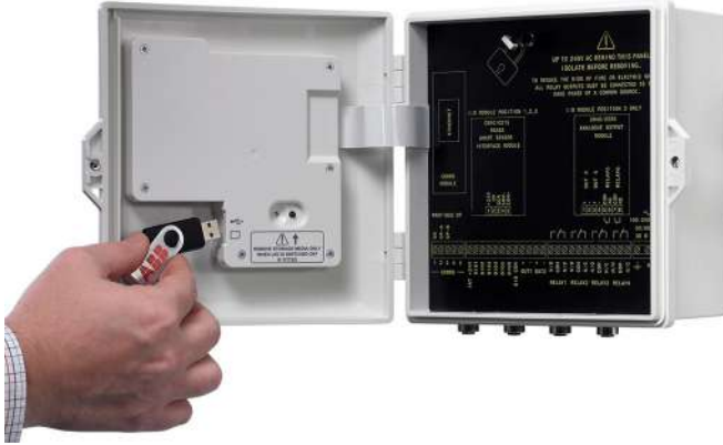
Fig. 3 SD card / USB stick access
