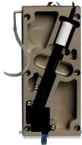
Figure 3 Electrode in temperature-controlled flow cell
