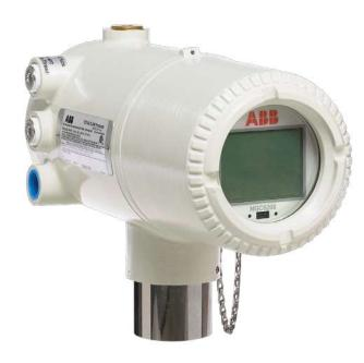
Using process chromatographic techniques, the columns are back flushed so that the NGC8206 measures a  $C_6+$  peak. Users may input the results of a comprehensive lab analysis that reflects the split or ratio of  $C_6$  through  $C_{10}$  components. This ratio can be used in subsequent analysis and energy calculations. Calculated values include:
