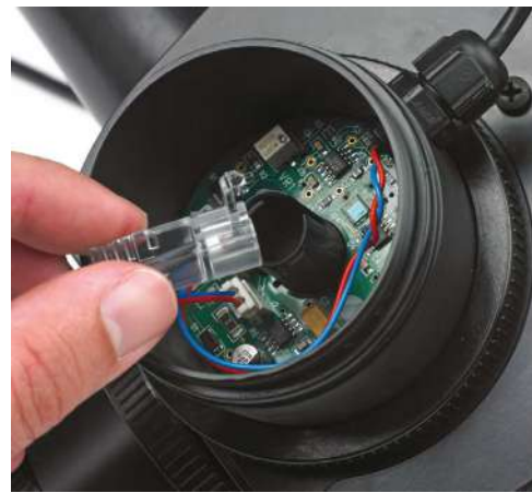
Figure 6 Replacing the light source
